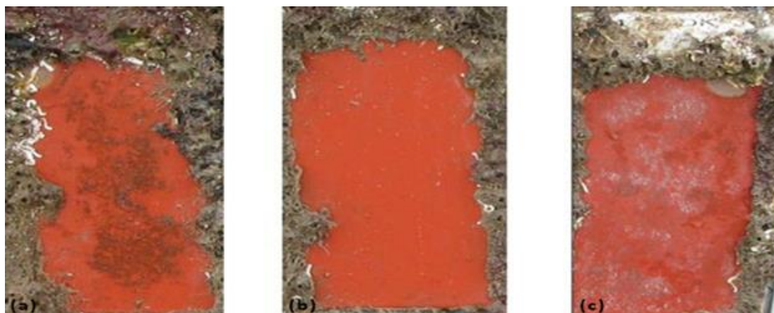
Figure 3.6 Mediterranean Sea antifoul coating trial with PDMS hydrogel enhanced FRC (a) compared to PDMS with Hydrogel (b) and Polymer (c)
