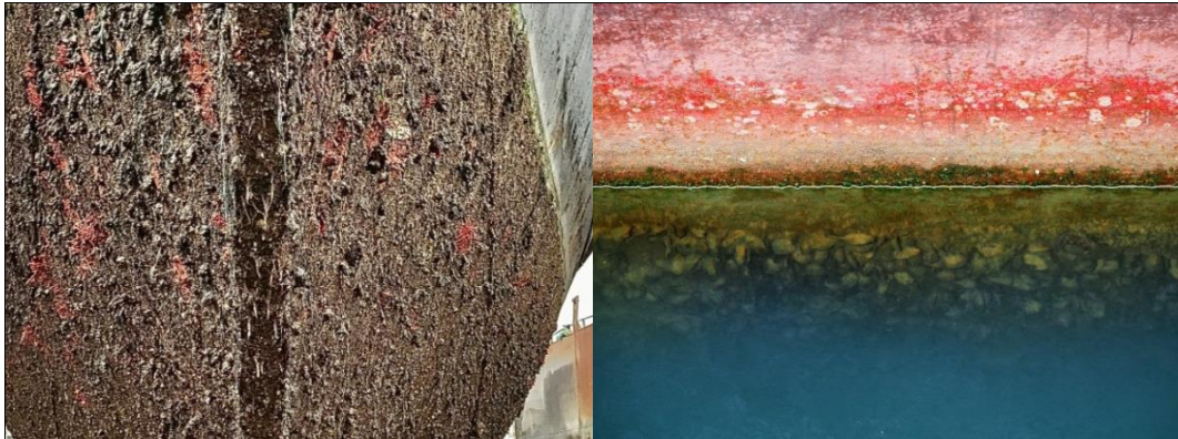
Figure 3.1 General biofouling and mussel / barnacle matrix on hulls
